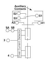
Module: Integrated wire termination. Terminals will accept PIN contact per M39029/1 - 101. Use insertion/extraction tool M81969/14 - 02.
