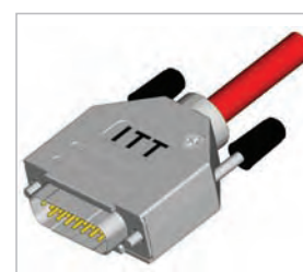
Assemble the other half (screwing force: 100-120 Ncm)
