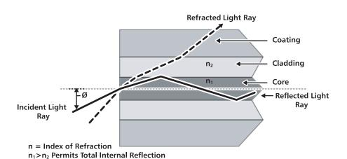
Figure 1. Core, Cladding, and Coating
