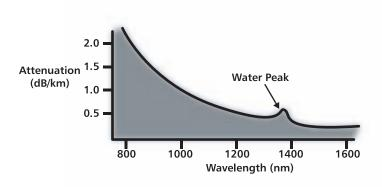
Figure 9. Typical Attenuation vs. Wavelength
