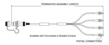
Harness Configuration: Connector to Connector
